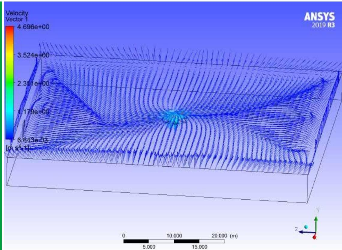
**7 airfoils is optimal ventilation result
