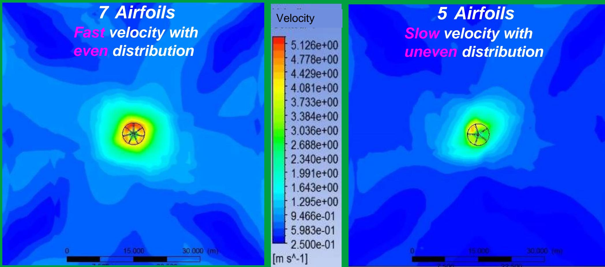
Powerful HVLS Fan Series10 (5M) the length of HVLS fan is 5m , away from ground is 1.4M to acquire velocity result
